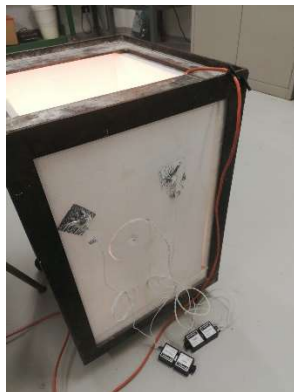
Fig.2 Hot box set-up, built at Building Physic laboratory of Politecnico di Bari
