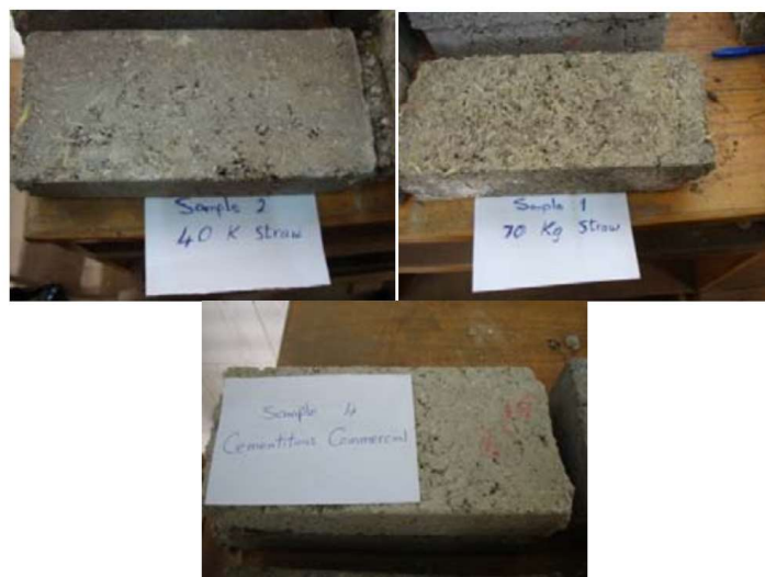
Fig.3 – Sample of concrete made with agro-waste (Garas et al., 2015)
