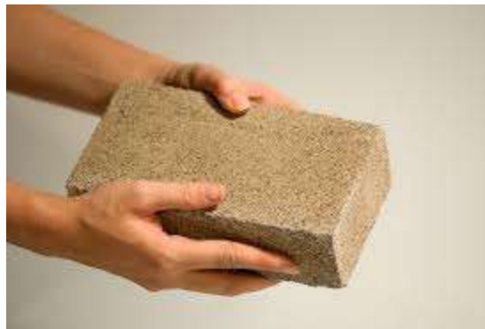
Fig.1 – Typical fired bricks realized with agro-waste ( KIIT Bhubaneswar, IIT Hyderabad Develop Bio-Bricks From Agro Waste - odishabytes )
