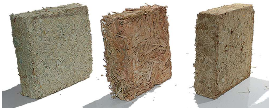
Fig.2 – Typical unfired bricks realized with agro-waste (Rautray et al. 2021)
