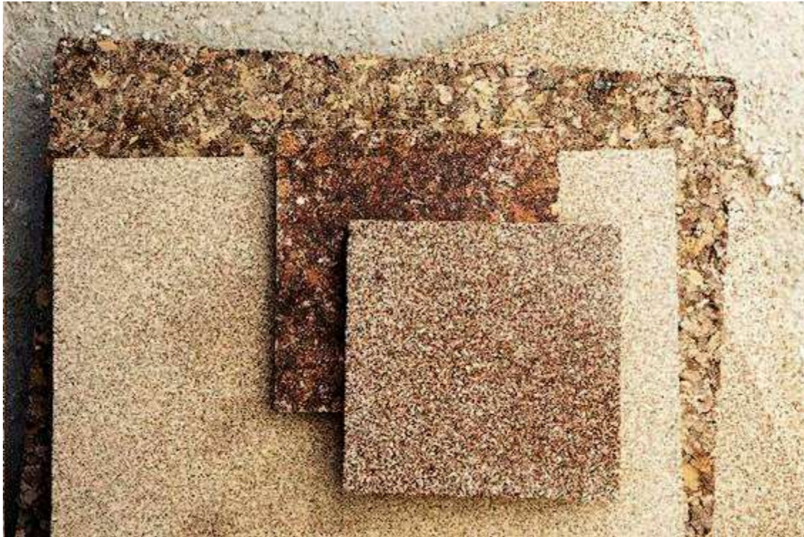
Fig.4 – Typical insulation panels made with agro-waste ( https://retaildesignblog.net/ )
