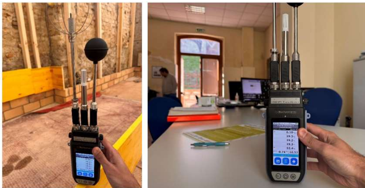
Fig.9 Monitoring equipment before and after the prototypes development (Microclimatic station HD32.3TC)
