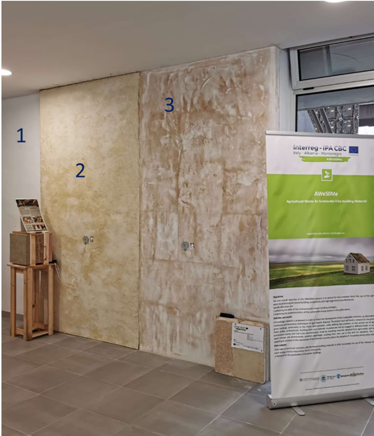
Fig. 3 Assessed wall, from left to right: 1) reference wall, 2) wall covered by lime-straw mix, 3) wall with lime plaster blocks.
