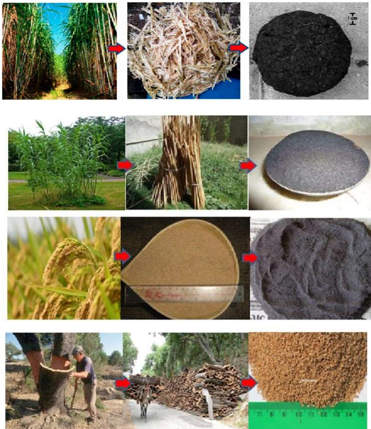
Fig.6 (From top to bottom) Processes to produce sugarcane bagasse ash, giant reed fibres and its ash, rice husk ash, cork processing aggregates. (Source: Prusty et al., 2016)
