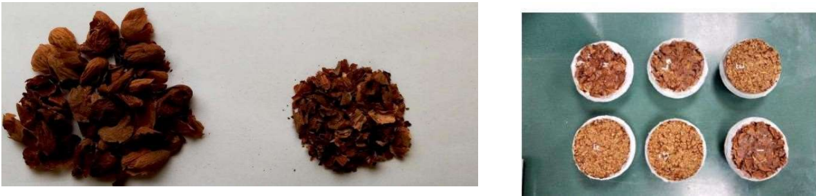
Fig.7 Sound sorption absorber made with almond skin waste (Liuzzi et al, 2020)
